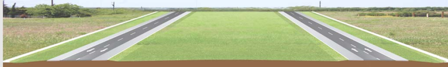
Phase 2: Add Second Two-Lane Frontage Road and Convert Phase 1 to One-Way Operation
